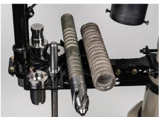
Cap Lifter with Hydraulic Arm and Table
